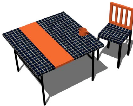
Figure 2 Connectedness demonstrated through a computational composite (the orange material) used for different purposes. When, for instance, the cup holds hot coffee the temperature of the back of the chair and stripe in the table will rise to ensure temperature equilibrium in the whole material.
